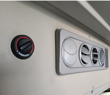
Impianto per riscaldamento in sosta supplementare System for stationary heating supplementary.
